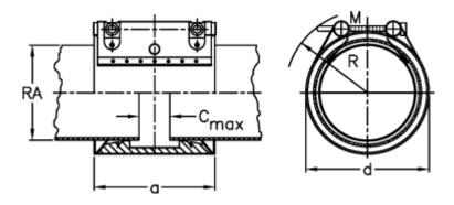
a = 62.4C max with insertion band = 8d = 70M (screw) = M8Nominal pressure (bar) = 16R = 90RA = 50.0RA min-RA max plastic = 49,5-50,5
